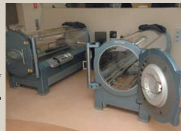
Two state-of-the-art hyperbaric chambers deliver 2.4 atmospheres of pressurized oxygen for optimum benefits.
